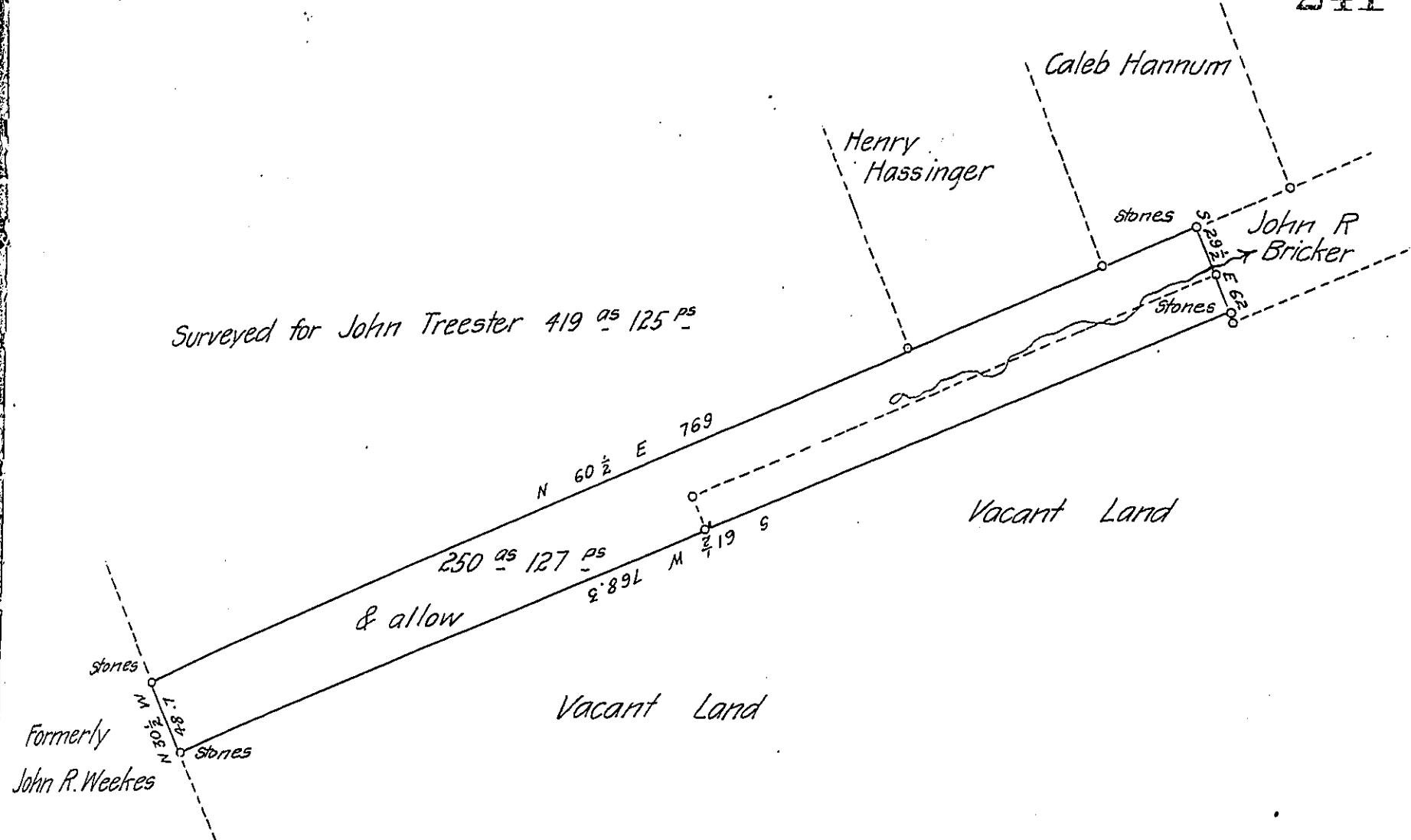
A draft of a tract of land situated in the Township of Armagh and County of Mifflin containing two hundred and fifty acres and one hundred and twenty-seven perches and allowance of six per cent for Roads &c Surveyed the 20<sup>th</sup> & 25<sup>th</sup> days of April, and the 10<sup>th</sup> & 11<sup>th</sup> days of May, 1892 in pursuance of a Warrant granted to John Locke dated the 12<sup>th</sup> day of Nov 1891
